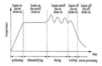
The above diagram represents a typical drying method for laundry dryers, belonging to  $\frac{D06F}{58/30}$  in which, during the drying process, the heater and the blower fan are subsequently turned ON/ OFF while the drum is rotated. It is noted that  $\frac{D06F}{58/30}$  relates to methods for treating the laundry
