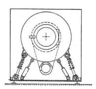
{Damping vibrations by displacing, supplying or ejecting a material, e.g. liquid, into or from counterbalancing pockets}
