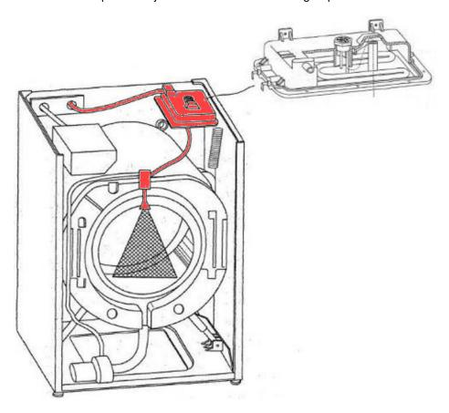
The drawing shows a washing machine provided with a steam generating equipment in the top-right rear corner. It is connected to the washing tub and can provide a spray of steam thereto. An enlarged drawing of the steam generating equipment is provided.
