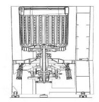
{Damping vibrations by displacing, supplying or ejecting a material, e.g. liquid, into or from counterbalancing pockets}
